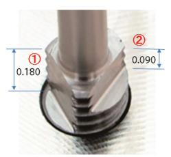
Ex) M10X1.5-6H Tolerance of pitch diameter is 0.180 pitch diameter value is around 0 as show on left photo. If target value is 75% of tolerance, threadmill should rotate larger.
