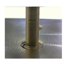
Work surface is over the 3rd notch (maximum Limit), about 1/8 of PD tolerance.
